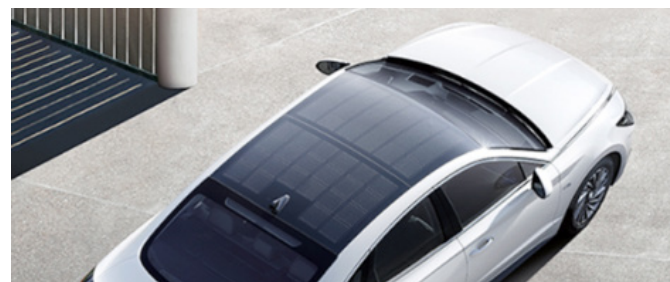
Vehicle-integrated Photovoltaic System
